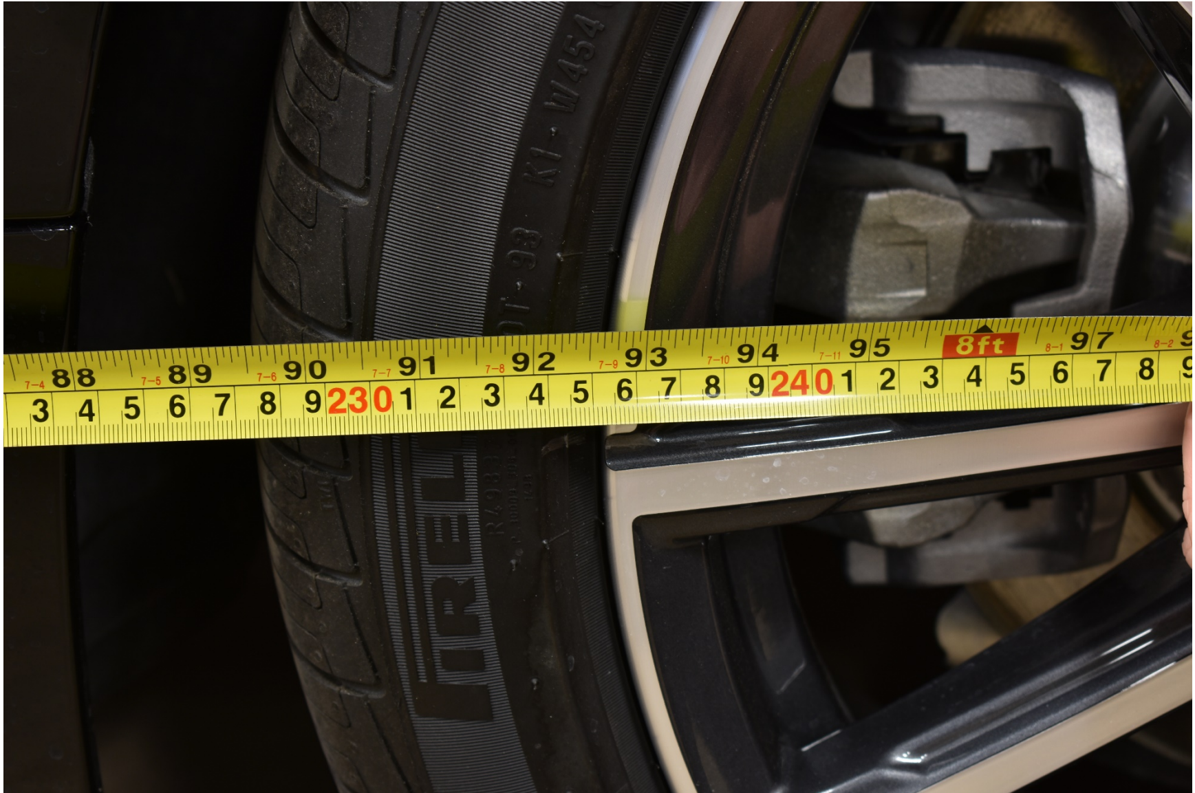
FIGURE 5.24 MEASURING VEHICLE LEFT SIDE WHEELBASE INSIDE EDGE TO INSIDE EDGE
